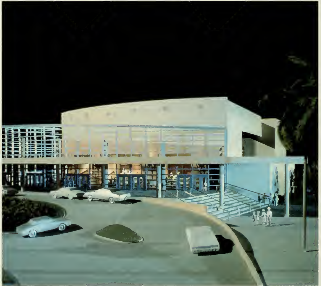
The model was created by laser-cutting plastic elements based on AUTOCAD drawing files. Photograph: Raul Pedroso, Solo Photography.
